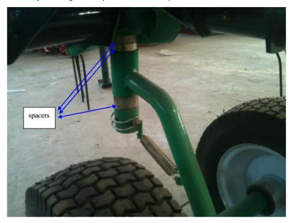
Fix the spacers previous than wheel sleeve, the working height is higher Fix the spacers below the wheel sleeve, the working height is lower 5 storage
