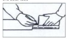
(3)Before cutting off, put rag into between safety cover and pipe not to come into sawdust
